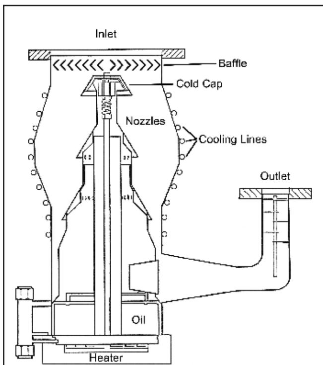
upward is caught by the vapor "skirt" above it and forced downward again. By continually forcing the air molecules downward, we create an area at the bottom of the pump that is higher in pressure than the top of the pump. In other words, when the pump is in operation the pressure is higher below each oil skirt than it is above that skirt. At the bottom of the pump, the pressure is high enough for the gas to be pumped out by a standard mechanical pump.
