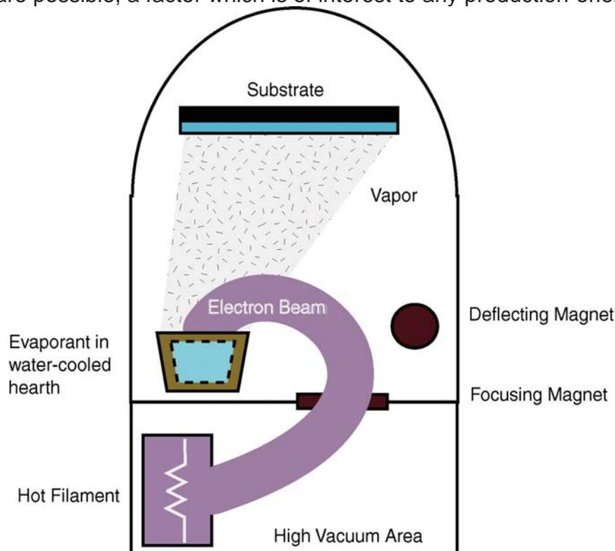
1 Filament is heated until it emits electrons. 2. Electrons leave the gun. 3. The beam is focused and bent by the magnet. 4. The beam plays upon the surface of the evaporant causing heat and vaporization. 5. The vapor condenses on the substrate surface.
