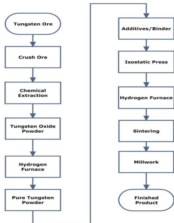
and use, but usually involves drawing through dies, or rolling through a mill, with annealing at various points. During the process the tungsten is further compacted, becoming more dense, and the crystal structure of the tungsten is manipulated in order to improve physical properties.
